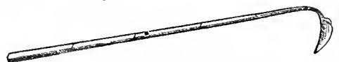
No. 2.—Length of handle, including iron socket, 4½ feet; handle of deal, and 1 inch diameter. The handle is marked in feet and inches. Length of blade, 4½ inches; breadth round, from edge to edge, 2 inches.
